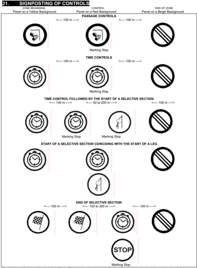
The minimum diameter of the panels is 70 cm. The drawing must be black. The panels will always be placed on the same side for the entire route of the Event.
